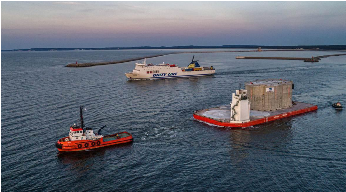
Fig. 10. Transport of caissons produced in the port of Świnoujście (source: https://www.aarsleff.biz )
