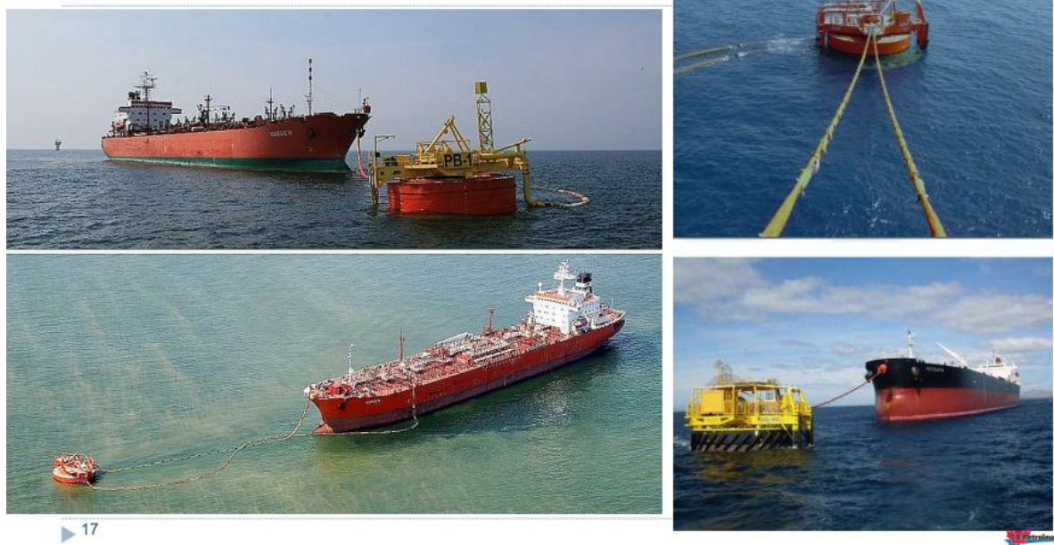
Fig. 13. Transport of crude oil using CALM buoys.
